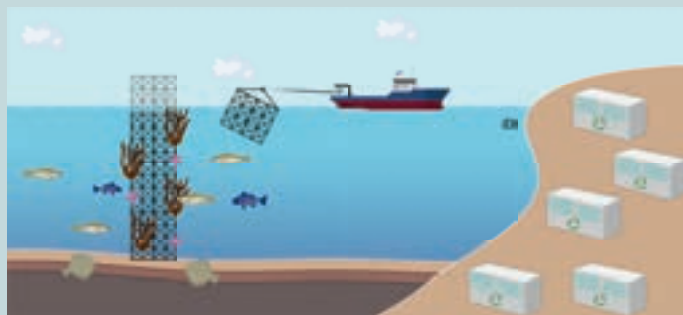
Removing the top of the foundation and taking it to shore for recycling
