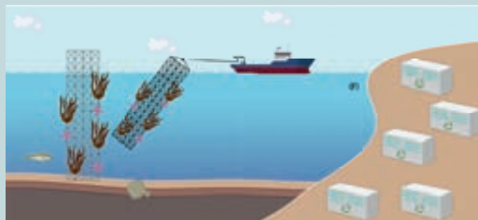
Complete removal of the foundation and recycling on land
