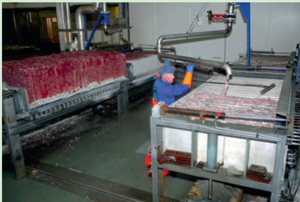
Vertical plate freezers can be conveniently filled from above. Here, for example, with shaft waste, which is deep-frozen in blocks until it is delivered to the fish meal factory.
