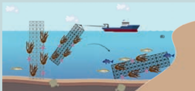
Transporting the complete foundation to a designated reefing area
