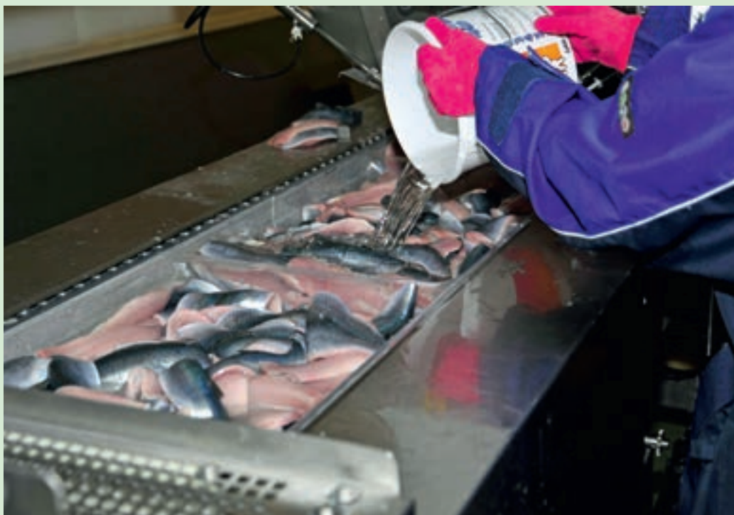
To reduce the risk of breakage of blocks made from very fatty fish products, they are often filled with water to stabilize them before deep-freezing.
