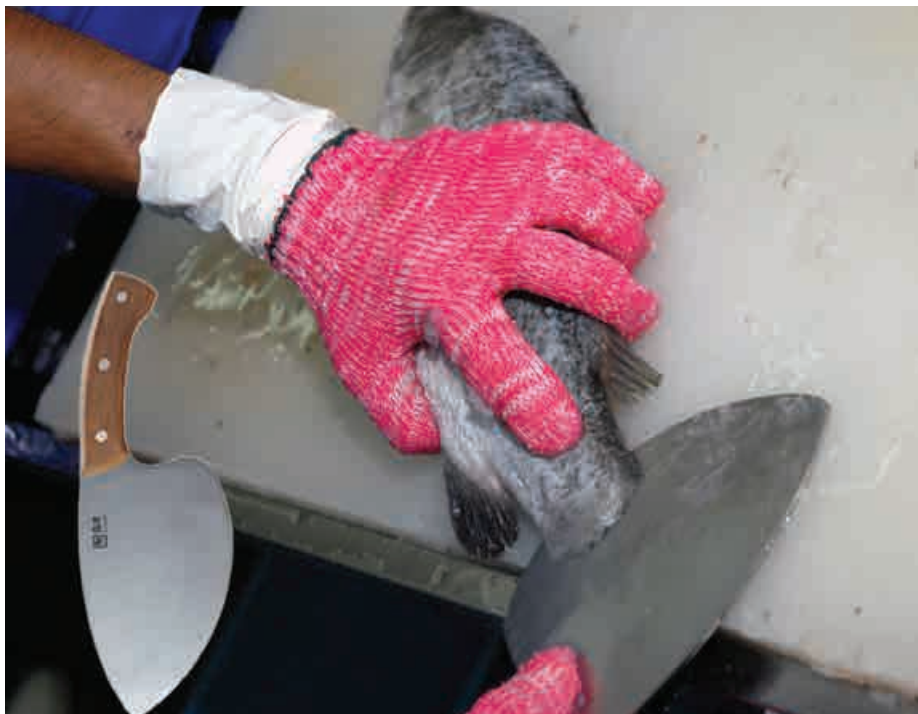
In Thai fish-processing plants, round knives are often used for filleting, with which semi-skilled employees can achieve high fillet yields after a relatively short period of training.
