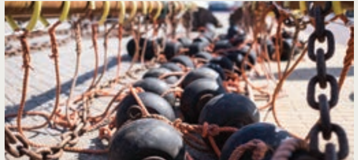
Rockhoppers are used in bottom trawling to help fishing nets navigate rough sea bottoms. They cause damage by crushing seabed organisms and altering marine habitats. The movement of rockhoppers stirs up seabed sediments, potentially releasing stored carbon and contributing to marine CO 2 emissions.
