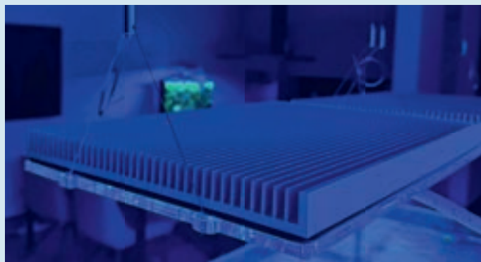
GNC lamps dissipate the heat generated with specially designed cooling ribs which maintain the operating temperature between 40 and 48 degrees C.
