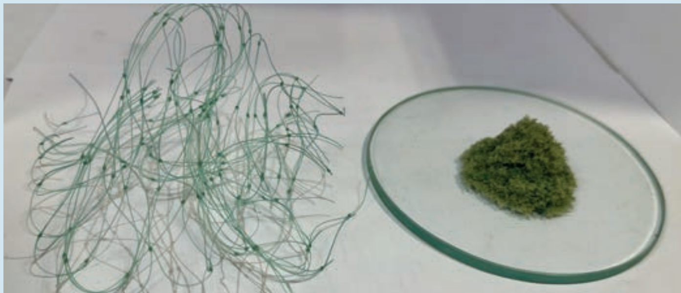
The nets are sorted and those that are identified as suitable are shredded to a fine powder (right). The powder retains the strength and flexibility of the original material.
