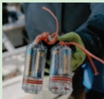
The PotLights are rated for a depth of 1,200 m, have a battery life of over 500 hours (800 when flashing), and are available in different colours.
