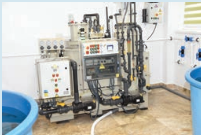
Renovated laboratories newly equipped with recirculation aquaculture systems that are used to study rainbow trout behaviour in saltwater.
