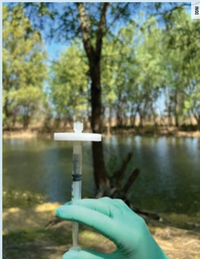
Using environmental DNA (eDNA) DDNI assesses the presence and abundance of aquatic species. Pictured, the process for filtering and preserving water samples.
