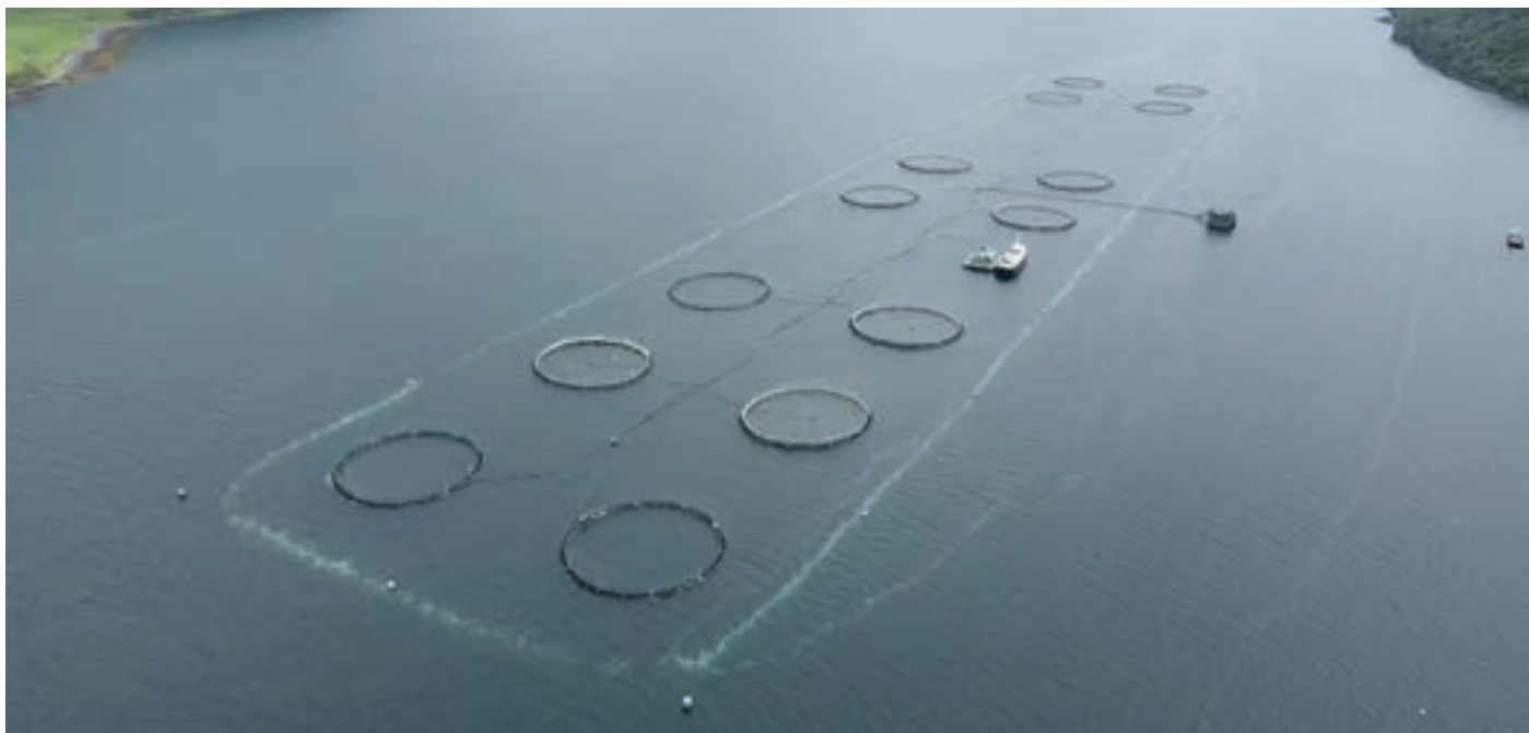
Bubble curtain technologies, like those developed by Mowi Scotland, create a protective barrier around salmon pens, helping to mitigate the damage caused by jellyfish blooms.
