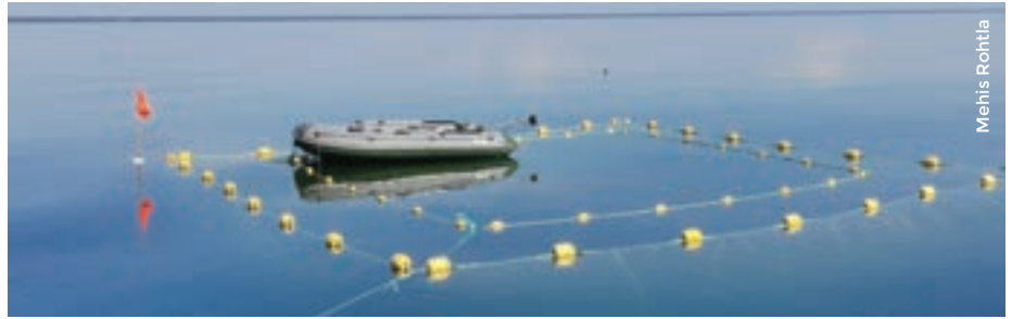
Once a herring shoal is located using sonar, researchers anchor the sound source and monitor the fish's movements by conducting transects—systematic paths taken by a survey vessel around the sound source.
