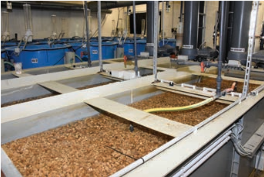
A recirculation aquaculture system allows HAKI researchers to conduct experiments with species cultivated intensively, such as African catfish.
