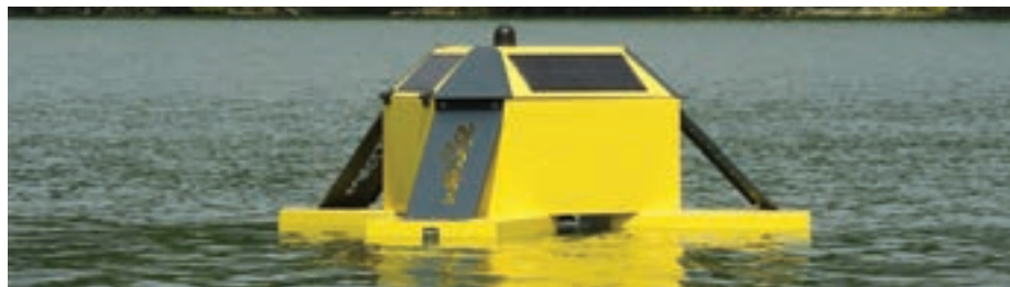
The buoys are equipped with sensors that monitor a range of values including temperature, oxygen content of the water, phytoplankton levels, pH and other critical parameters (blue-green algae, ammonia, etc.).
