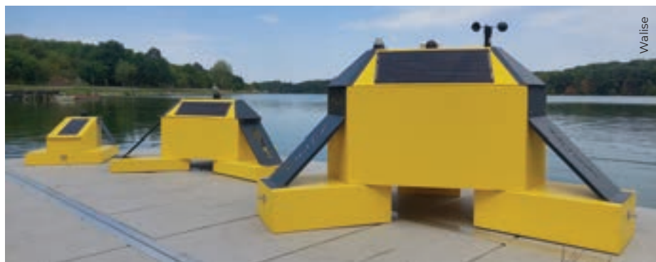
Three of the company's models: from left, the CMU is for fixed depth measurements at 40 cm making it ideal for shallow lakes and rivers; the Shallow Measurement Unit (SMU) is used in water around 2 m deep; while the Profiling Measurement Unit (PMU) can be deployed in water up to 20 m deep.
